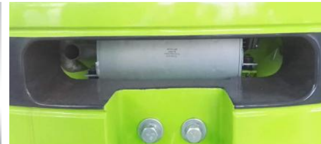
Mid exhaust pipe set, effectively avoiding the problems caused by low exhaust dust problems
